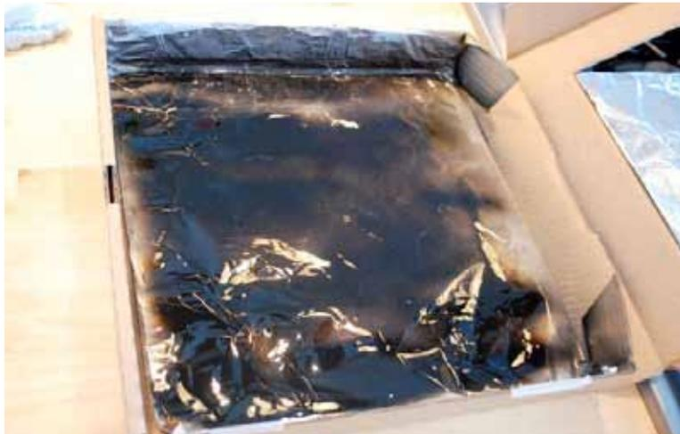
8. At this point, you may wish to have students construct an insulating layer in the bottom of their solar cooker. This step is optional, but it will help the cooker retain heat. To do this, place insulating material on top of the layer of black aluminum foil. Insulating material can be shredded paper, wadded cotton balls, or pieces of rigid foam. Then repeat Step 7 so that the insulating material is covered with another layer of aluminum foil and painted black.
