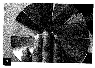
Cut the tail off the plastic pen cap with the cutting pliers. Then push the tip of the pen cap through the center hole of the pie plate. Use the screwdriver to expand the hole if necessary. Set this aside.
